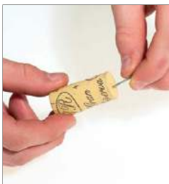
Pic. 11: A Cork with a Magnetic Needle
